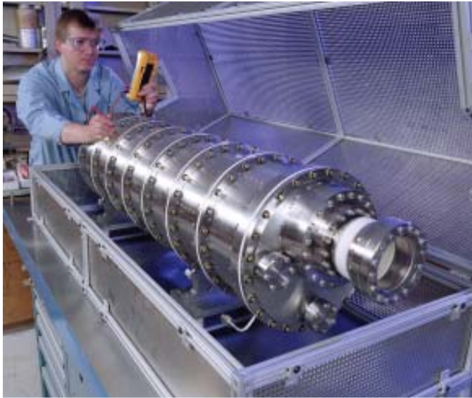
GAS CATCHER – Argonne physicist Guy Savard examines a gas catcher cell being installed for the CARIBU updated to the Argonne Tandem Linear Accelerator System. The cell provides a new way to generate intense beams of short-lived, exotic nuclear isotopes for basic research in nuclear physics and other sciences.
